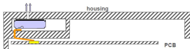
Case n°4: Create closed box - Contacting with contact spring
